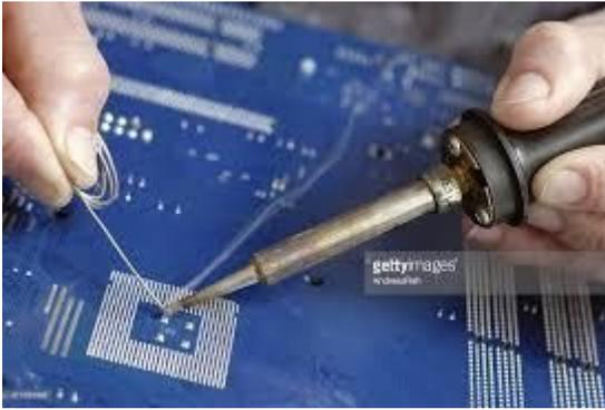
Soldering is a process in which two or more metal items are joined together by melting and then flowing a filler metal into the joint—the filler metal having a relatively low melting point. Soldering is used to form a permanent connection between electronic components.
